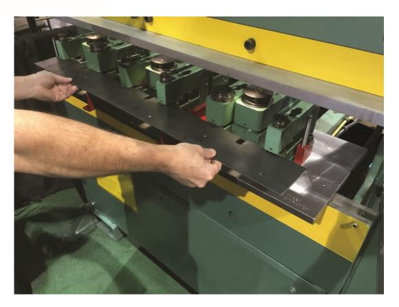
Shown above are UniPunch "B" units mounted in a press brake with a limited opening between the press ram and bed. Keyed mounting templates are available for positioning "B" units and gauges to produce accurate parts with each stroke of the press.
