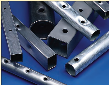
Tube Punching – Round or Square Tubing
