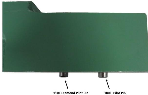
Using the same process as above, install the diamond pilot pin (P/N 1101) into the second hole making sure a point of the diamond shape faces the front of the unit.
