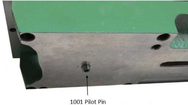
**Die Removal for the 2820 Die:** To remove the die, loosen the die set screw (P/N 91350 5/16-18 x 3/8) in the front of the holder and, if necessary, push the die up out of the holder from the slug chute.
