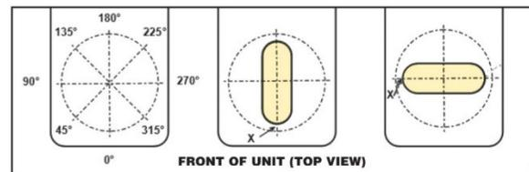
Extract the punch and apply a thin coat of lubricant (e.g. P/N 8007 Molykote® type G-N metal assembly paste) to the punch body. Put the punch and head assembly through a stripping spring (P/N 2140) and into the guide in the same shape orientation as the die. Push the retainer pin (P/N 2180) through the hole that is parallel to the flat on the punch until it clips on to the guide collar.
