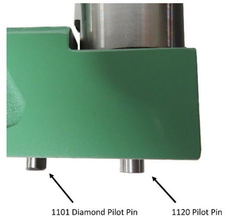
**Pedestal Die Removal:** To remove the shaped pedestal die (P/N 2126), first loosen the guide retainer (P/N 1018) on the upper arm of the unit to allow the guide to lift up. Use a hex key wrench to loosen and remove the 1120 pilot pin and lock washer from the lower arm of the unit and lift the pedestal die up and out of the unit.
