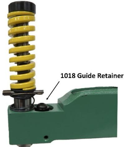
**Punch Installation:** First be sure the punch and head assembly (P/N 2016) will fit in the die by inserting it in the same intended orientation as the die and dropping it through the guide (without the stripping spring) and into the die. Visually look to see that the die clearance is even all the way around. If the die clearance is uneven, contact UniPunch.
