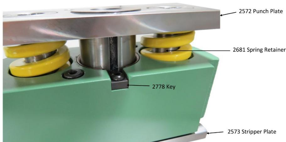
Assemble the (2) stripping springs (P/N 2540) into the two larger pockets on the top of the upper arm. Then put the punch plate (P/N 2572) on top of the springs and drop the (2) spring retainers (P/N 2681) down thru the center of the holes on the punch plate and down thru the center of the stripping springs. Then insert the (2) stripper bolts (P/N 2682) down thru the spring retainers and tighten into the stripper plate.
