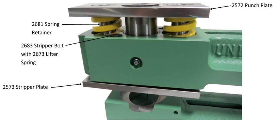
Assemble the (2) stripping springs (P/N 2540) into the two larger pockets on the top of the upper arm. Then put the punch plate (P/N 2572) on top of the springs and drop the (2) spring retainers (P/N 2681) down thru the center of the holes on the punch plate and down thru the center of the stripping springs. Then insert the (2) stripper bolts (P/N 2682) down thru the spring retainers and tighten into the stripper plate.
