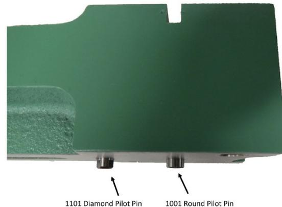
Using the same process as above, install the diamond pilot pin (P/N 1101) into the second hole making sure a point of the diamond shape faces the front of the unit.
