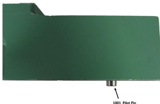
**Block Die Removal:** To remove the block die (P/N 2621), turn the unit on its side and unscrew the two S.H.C.S (P/N 91029) from the lower arm. Then lift the block die up out of the unit.
