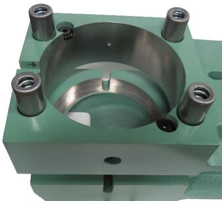
Assemble the (4) lifter springs (P/N 1470) into the four pockets on the upper arm of the holder. Then assemble the (4) spring cages (P/N 6043) on top of the lifter springs as shown in the picture on the left. Insert the (2) guide retainers (P/N 1018) into the two corner pockets of the upper arm of the holder, making sure the flat on the guide retainer is facing the center of the guide bore of the holder.
