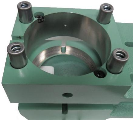
Assemble the (4) lifter springs (P/N 1470) into the four pockets on the upper arm of the holder. Then assembly the (4) spring cages (P/N 6043) on top of the lifter springs as shown in the picture on the left. Insert the (2) guide retainers (P/N 1018) into the two corner pockets of the upper arm of holder, making sure the flat on the guide retainer is facing the center of the guide bore of the holder.
