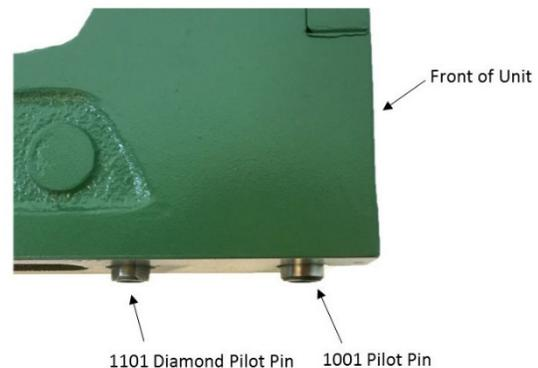
Using the same process as above, install the diamond pilot pin (P/N 1101) into the second hole making sure a point of the diamond shape faces the front of the unit.
