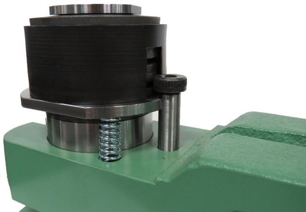
Assemble guide assembly into holder. Insert stripper bolt (P/N 91420) into upper arm of holder. Align the cut-out pocket on the spring guard with the stripper bolt and tighten bolt.
