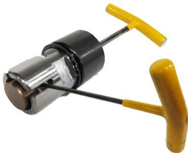
top of the guide. Insert the punch screw thru the punch driver and by hand engage a few threads into the punch. Put the punch and guide assembly into a soft jaw vice and tighten the vice just enough to prevent the guide from spinning while you tighten the screw. Use a hex key wrench to tighten the punch screw.
