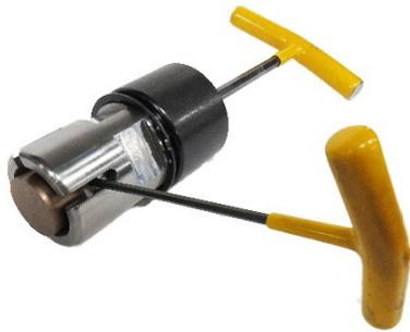
hole in the punch. Put the punch and guide assembly into a soft jaw vice and tighten the vice just enough to prevent the guide from spinning while you tighten the screw. Use a hex key wrench to tighten the punch screw. **Important:** tighten the punch screw until the punch driver is tight against the punch so that during punching operation the punch driver is what engages the punch and not the
