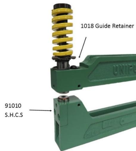
**Punch Installation:** First assemble a punch head (P/N 2171) onto a punch (P/N 2111) being sure the counter bore in the flange of the punch head faces the retaining ring, creating a punch and head assembly (P/N 2110). When assembled correctly, the top of the punch head is flush with the top of the punch.
