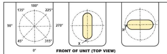
Extract the punch and apply a thin coat of lubricant (e.g. P/N 8007 Molykote® type G-N metal assembly paste) to the punch body. Put the punch and head assembly through a stripping spring (P/N 2045) and into the guide. According to the orientation, push the retainer pin (P/N 2180) through the hole that is parallel to the flat on the punch until it clips on to the guide collar.
